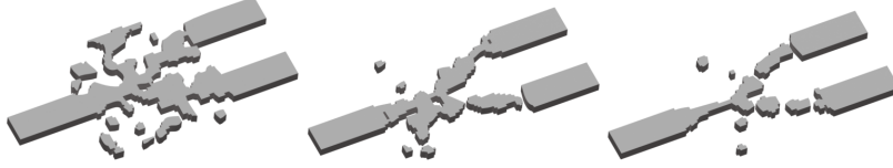
Figure 6: A three-dimensional rendering of the optimized design. Silicon is shown in grey and light enters the optimized device from the input waveguide on the left-hand side (port 1) and exits via one of the two output waveguides (port 2 and port 3) on the right side. There are three optimized devices with different volume fraction: (left) \gamma = 0.474 , (middle) \gamma = 0.3 and (right) \gamma = 0.2 .
